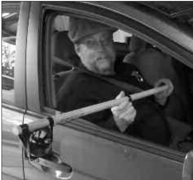
Lynn prepares to record calibration readings on one of his homemade anemometers.
