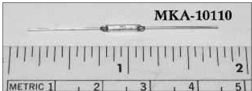
This 10mm magnetic reed switch, acquired on eBay for less than two dollars, can switch up to 15W in about 0.001s. Normally open, the switch will close when a magnet is brought sufficiently close.
