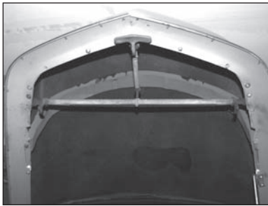
The red rubber seal , as fitted to the hood of Josh Malks's Moonshadow . (Mod3)
