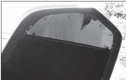
Ray Simpson's hood baffle . Notches were required to clear the hood latch arms and return spring. (Mod4)
